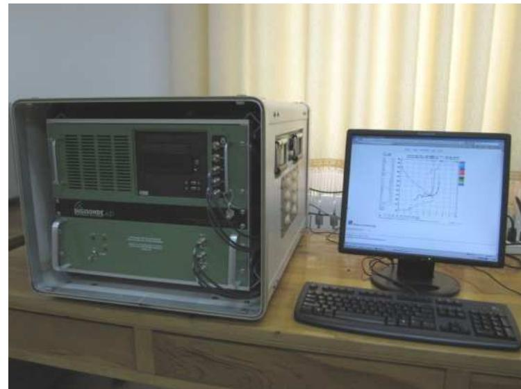
**Ionosonde to get ionospheric parameters and electron profile from ionogram**
