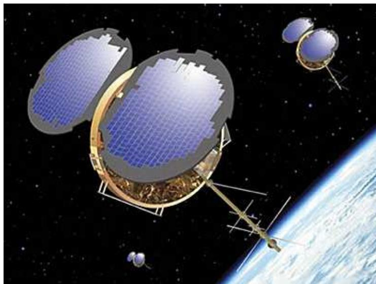
**COSMIC satellites to get ionospheric electron profile by GPS radio occultation**
