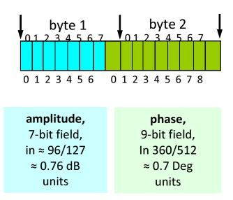
One databin for each frequency, polarization, height, antenna, and Doppler
