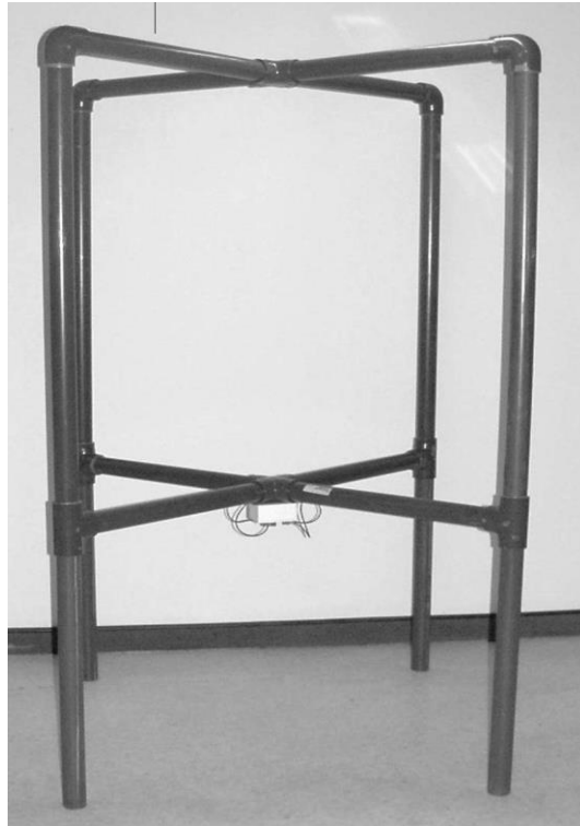
Figure 1-3: Turnstile Receive Antenna with Attached Preamp Module
